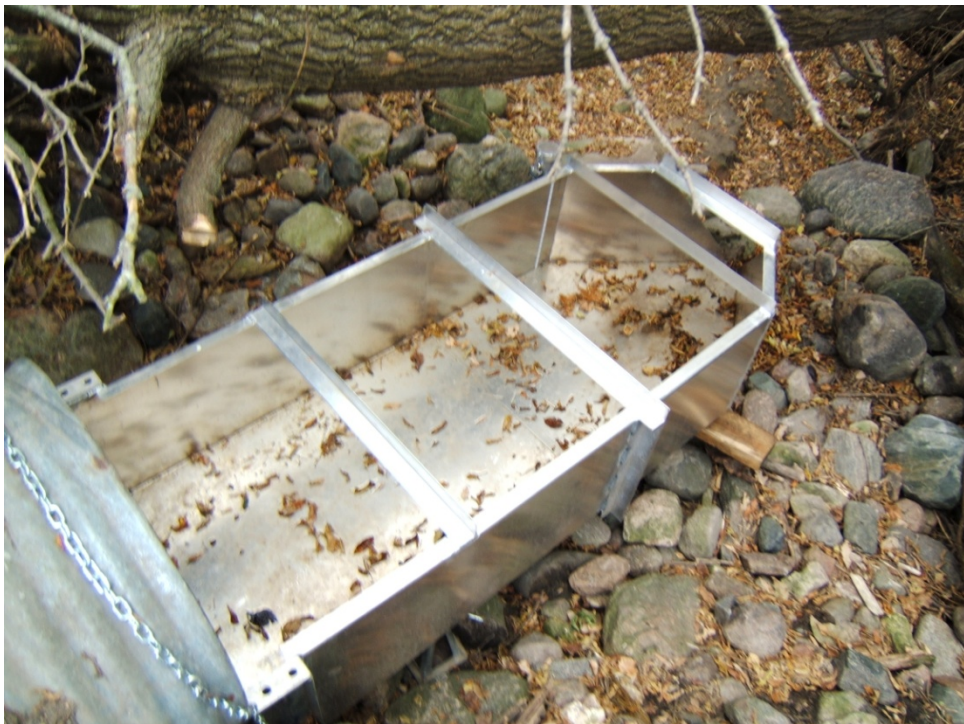
Figure 19. H-Flume on Downstream End of Yaggie 2 Culvert
