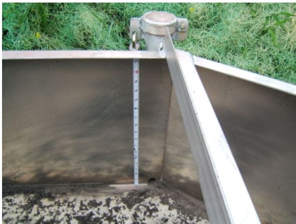
Figure 9. Stilling Well and Gauge on Bachand Surface H-Flume
