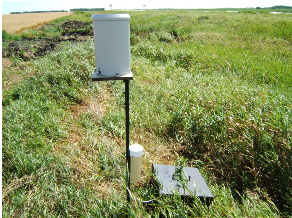
Figure 17. Rainfall and Barometric Pressure Monitoring Equipment at the Bachand Site
